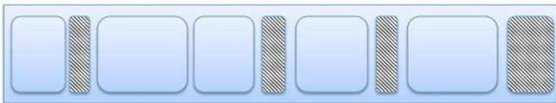
Fragmented memory before compaction
